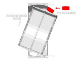
5. Rotate the inner race and the first track of roller in opposite direction so the other roller track is just exposed at the upper edge and a roller can be placed in the track.
